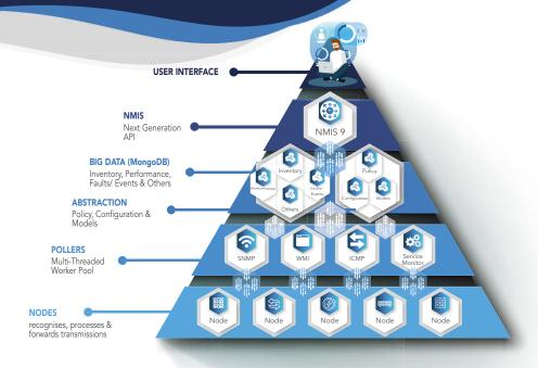
**NMIS (Network Management Information System)** is a complete network management system which assists with fault, performance and configuration management, providing performance graphs and threshold alerting as well as highly granular notification policies with many types of notification methods. NMIS monitors the status and performance of an organization's IT
